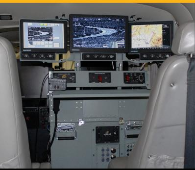
The Battlestation is a self-contained rollon-roll-off (RO/RO) operator workstation configured for Armed ISR operations.
